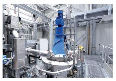
Fig. 2: The strength of short path distillation is that it is gentle on unsaturated fatty acids and yet provides effective purification. (Photo®: Nutriswiss)
